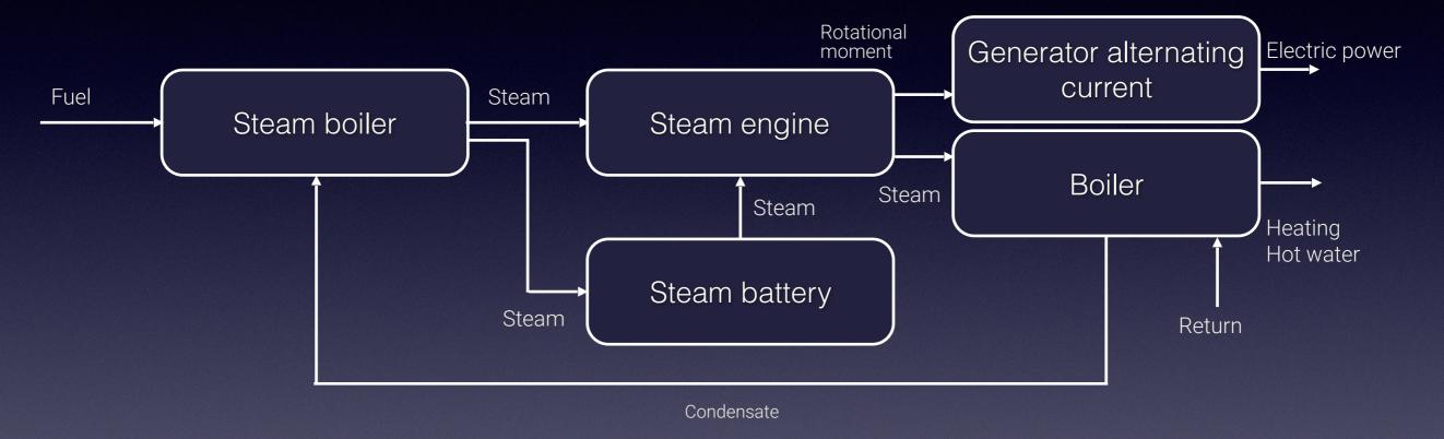
Schematic diagram of the operation of the solid fuel boiler «TurboRapid®»
